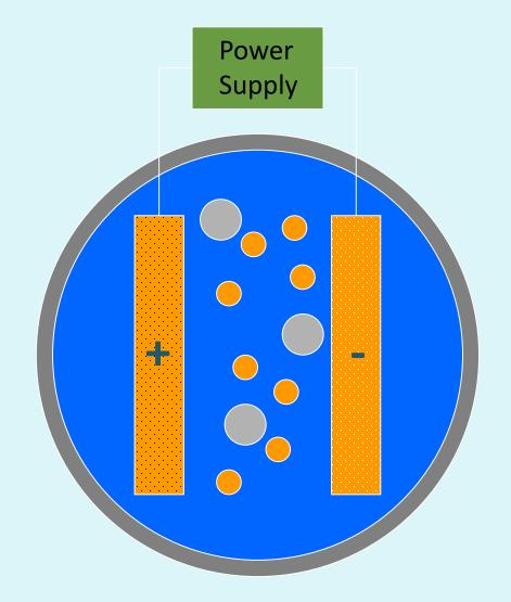
The ionization chamber contains sets of pairs of electrodes made from a calibrated copper-silver alloy.
